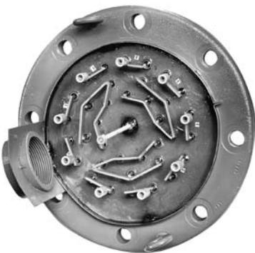
**Large Diameter Elements** - Elements measure .475" O.D., providing extra electrical insulation for superior dielectric strength. As a result, elements are suitable for line voltages up to 600 volts. At the same time, uniform heat transfer from coil to sheath is assured by compacting the insulation in high pressure rollers, then repressing all bends to insure insulation integrity in this critical area. Copper sheathed elements are silver soldered to the flange; all other materials are welded.
